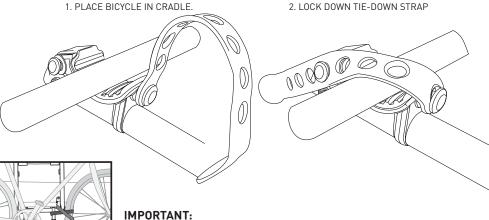
SECURE FRONT WHEEL OF INSIDE BICYCLE WITH EXCESS BOTTOM STRAP, OR ADDITIONAL STRAPS TO PREVENT WHEEL FROM COMING INTO CONTACT WITH VEHICLE.
