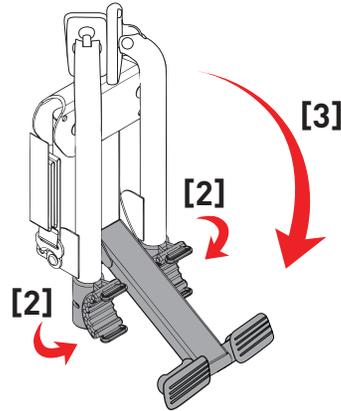
4. ROTATE BOTH TOP FEET DOWN BY 90 DEGREES TO OPEN, FULLY ENGAGING PINS
