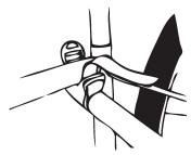
3. USE 70" STRAP (NOT INCLUDED) TO PULL ALL BICYCLES TOGETHER AROUND BOTTOM BRACKETS. STRAP SHOULD ALSO SECURE WHEELS
