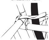
4. USE 70" STRAP (NOT INCLUDED) TO PULL ALL BICYCLES TOGETHER AROUND BOTTOM BRACKETS. STRAP SHOULD ALSO SECURE WHEELS.
