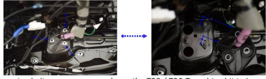
Step 5: The two wing bolts are now exposed, use the T20 / T30 Torx drive bit to loosen the bolts (not remove, just loosen). Just for the first few rotations, make sure to apply pressure toward the bolt while turning. Over time, these bolts can become rusted so you want to ensure that there is a good seat for the torx driver bit. Do this for both the left and the right side.
