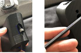
Step 9: (Optional, and only applicable to 60mm and 100mm extenders) You may choose to use the provided cylindrical rear cover piece to cover the rear bolt head from environmental debris
