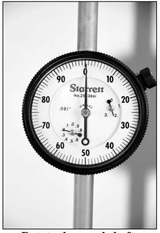
Rotate the crankshaft clockwise .200".
