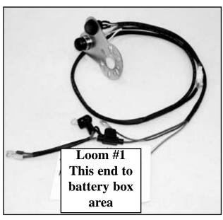
The "on" button with a light plugs into wire loom part 1. The "on" button along with the starter button, mount in the switch bracket. Then attaches to the steering wheel. The blue and white wires on loom 1 attaches to the starter button. The other end of loom 1 goes to the battery box as shown in #15 of the fitting instructions.
