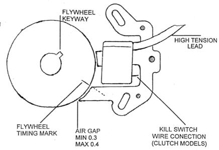
(THIS IGNITION DOES NOT REQUIRE AN EXTERNAL MODULE) IMPORTED & DISTRIBUTED BY ST GEORGE KART CENTRE P/L
