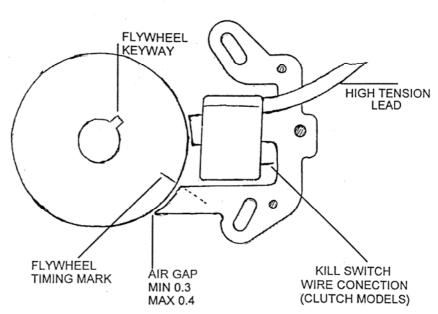
(THIS IGNITION DOES NOT REQUIRE AN EXTERNAL MODULE) IMPORTED & DISTRIBUTED BY ST GEORGE KART CENTRE P/L
