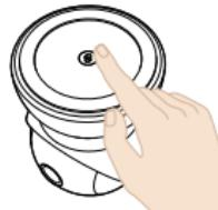
Press and hold the **Pair Button** on the bottom of the camera until a beep is heard.
