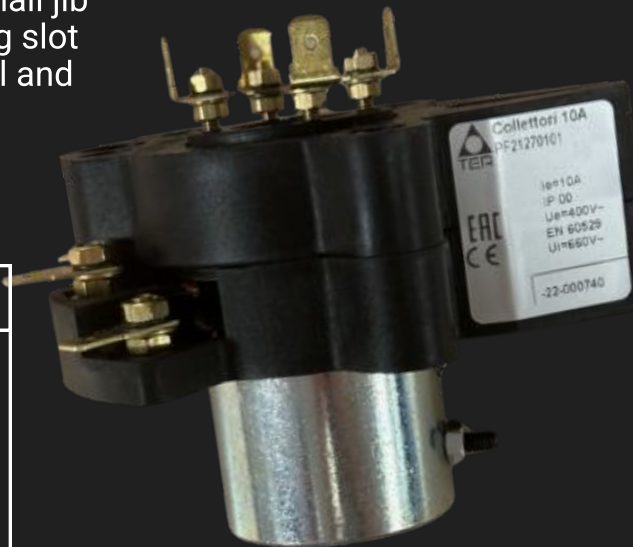
PF21270101 10 Amp Slip Ring with 4 Circuits and 40mm flange
