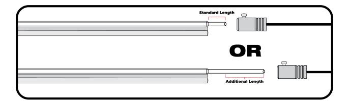
3. Insert the inner fiber optic cable sections into their corresponding outer tubing sections, as demonstrated in the diagram below.
