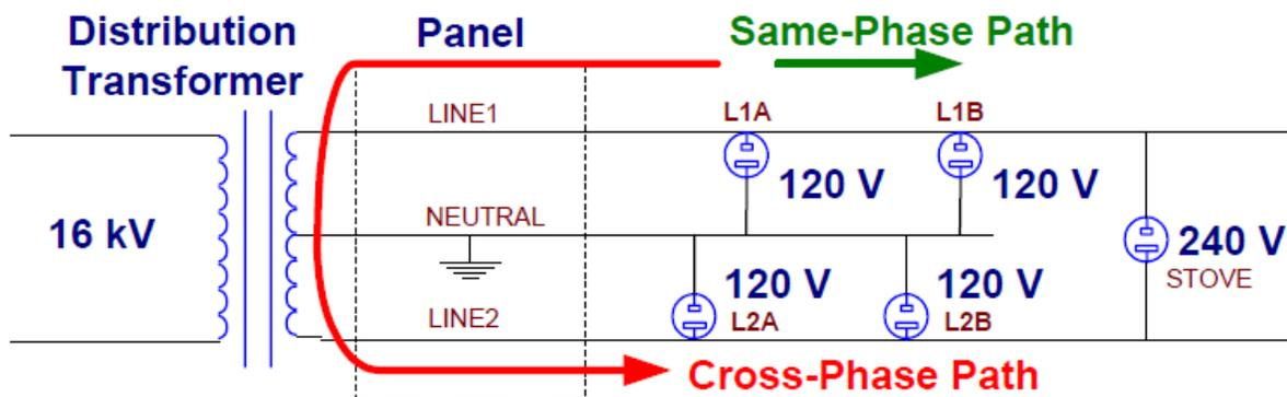
Figure 3. Electrical outlets in a typical North American home
