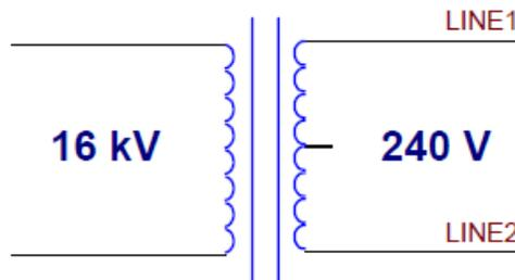
**Figure 1. Transformer for a typical North American home**
