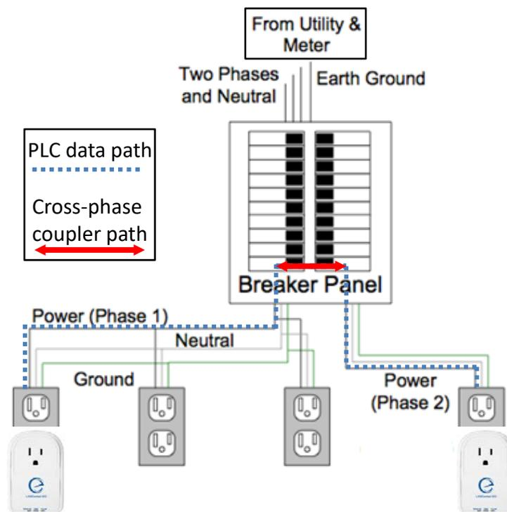
Figure 6. The cross-phase coupler path
