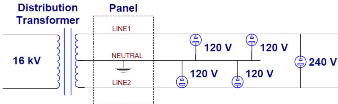
Figure 2. Electrical wiring in a typical North American home
