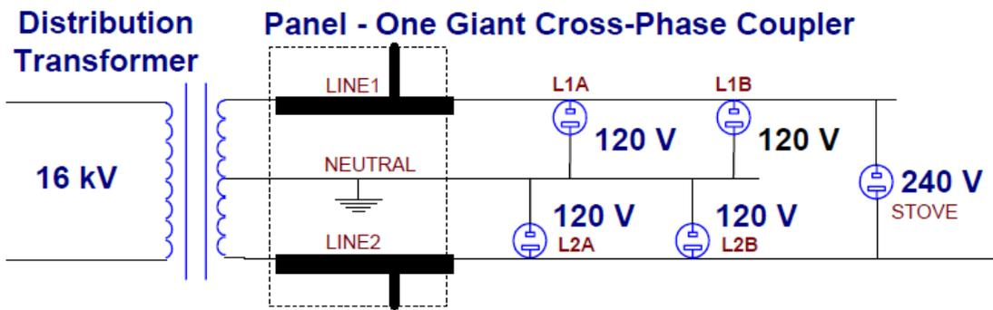
Figure 5. The electrical panel acts as a cross-phase coupler
