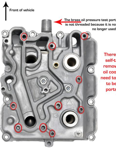
There will be ten (10) self-tapping screws removed from the old oil cooler that you will need to reuse. They are to be seated in the ports as marked on the image.
