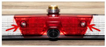
Remove the screws and seperate the adapter from the lens. You will see a slight indentation. Use these markings as a guide to carefully file the lens housing for clearance.
