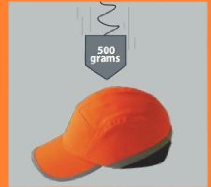
A penetration test is carried out at lower energy and involves a 500g striker being dropped from a height 500mm onto the bump cap fitted to a fixed headform.
