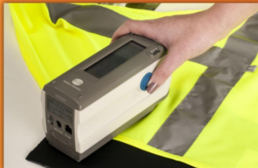
A spectrophotometer is used to check the chromaticity - "colour intensity" - of fabric. We use this to ensure every roll of fabric meets the requirements of EN ISO 20471 and RIS-3279-TOM.
