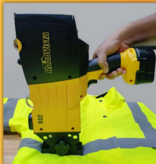
To evaluate the effectiveness of retroreflective tape, a retroreflectometer is employed. Every roll of tape is put through testing to make sure it satisfies and beyond industry standards. The coefficient of two rotating angles is measured by the retroreflectometer. According to EN ISO 20471, the reading must be at least 400 (cd/lx.m<sup>2</sup>); however, at Portwest, we demand a value of at least 330 (cd/lx.m<sup>2</sup>).
