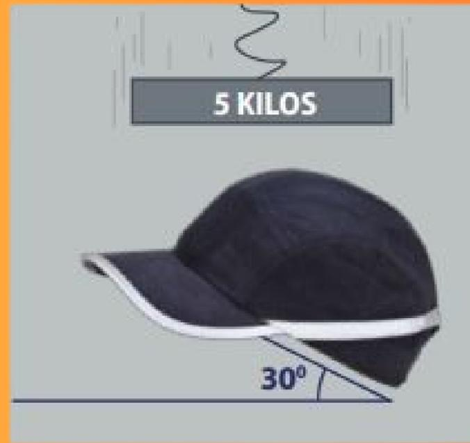
To achieve the impact test, a 5 kg fl at striker is dropped onto the bump cap from a height of 250 mm, with a maximum allowable transmitted force of 15 kN. Impacts are carried out on the front and rear of the bump cap, with the headform tilted at 30° and 60° to reflect the nature of any impacts likely in use.
