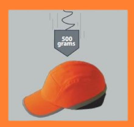
A penetration test is carried out at lower energy and involves a 500g striker being dropped from a height 500mm onto the bump cap fitted to a fixed headform.
