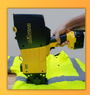
To evaluate the effectiveness of retroreflective tape, a retroreflectometer is employed. Every roll of tape is put through testing to make sure it satisfies and beyond industry standards. The coefficient of two rotating angles is measured by the retroflectometer. According to EN ISO 20471, the reading must be at least 400 (cd/lx.m2); however, at Portwest, we demand a value of at least 330 (cd/lx.m2).
