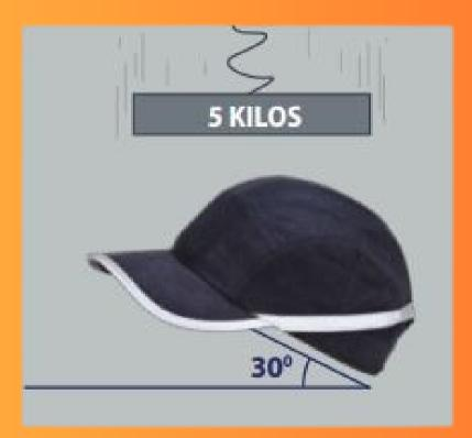
To achieve the impact test, a 5 kg fl at striker is dropped onto the bump cap from a height of 250 mm, with a maximum allowable transmitted force of 15 kN. Impacts are carried out on the front and rear of the bump cap, with the headform tilted at 30° and 60° to reflect the nature of any impacts likely in use.
