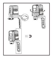
Make sure the laser screw hole is aligned with stand screw arbor and ensure the laser direction is correct, rotate the stand knob and the laser will be fully assembled with stand.
