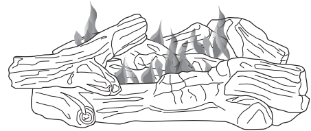
Figure 33 - Correct Flame Pattern with Control Knob Set to High Flame.
