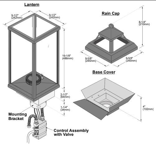
**NOTE**: Side clearances are measured from the glass – Top clearances are measured from the glass frame.
