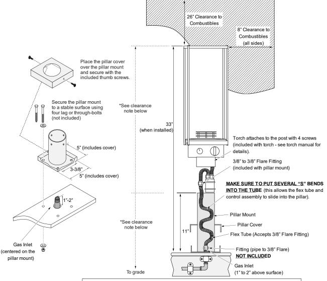
\*NOTE: The distance from ground level to the top of the Torch shall be a minimum of 7' (2.1m) where installed within 2' (0.6M) of public walkways (e.g.: sidewalk, shared walkway between two homes, or pathway in commercial applications). Lesser clearances shall be permitted to be used only where acceptable to the authority having jurisdiction.
