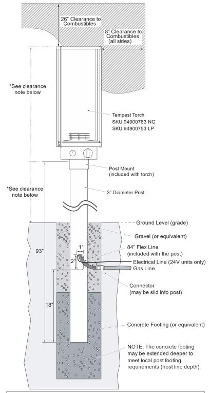
\*NOTE: The distance from ground level to the top of the Torch shall be a minimum of 7' (2.1m) where installed within 2' (0.6M) of public walkways (e.g.: sidewalk, shared walkway between two homes, or pathway in commercial applications). Lesser clearances shall be permitted to be used only where acceptable to the authority having jurisdiction.
