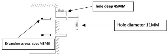
Step 4: Fix adjusting bracket into wall with expansion screws.
