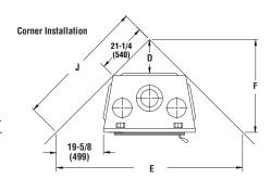
Combustible materials can NOT be used in the space directly above the fireplace. Do not fill the space above the fireplace with any material (Except the wood framing)
