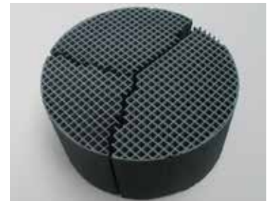
Photo #3 Thermal Cracks
