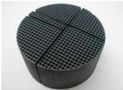
Photo #4 Mechanical Cracks
