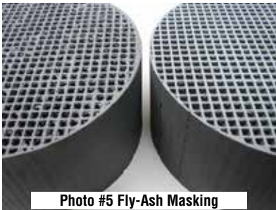
Photo #5 Fly-Ash Masking
