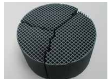
Photo #3 Thermal Cracks
