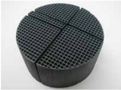
Photo #4 Mechanical Cracks
