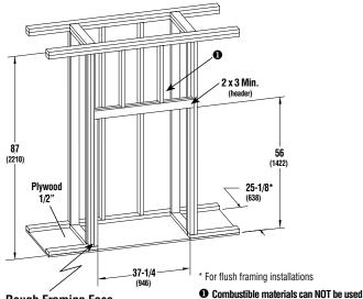
**Rough Framing Face** (dimension includes finish material inside framing, if any)
