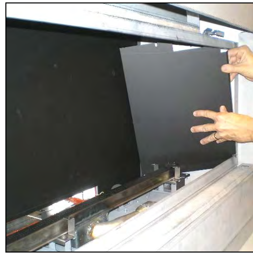
Insert Back Liner. Tilt Side Liners into place and attach to firebox with Screws removed from sides of firebox. Replace all components.
