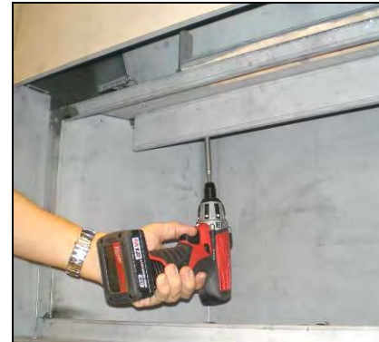
Remove False Bottom, Pilot Cover, and Upper Baffle.
