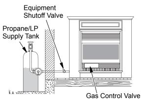
Figure 26 - Checking Gas Joints (Propane/LP Only)
