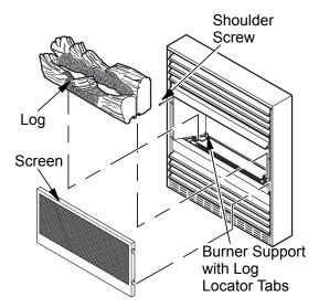
Figure 32 - Installing Log and Screen
