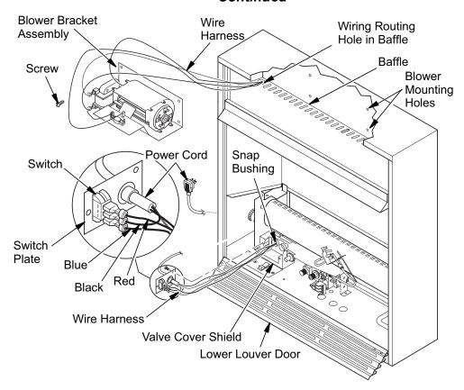
Figure 16 - Installing Blower Bracket Assembly
