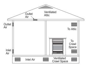
Figure 5 - Ventilation Air from Outdoors
