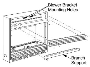
Figure 15 - Removing Top Louver and Branch Support
