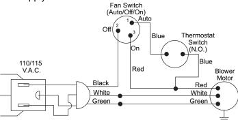
Figure 19 - Wiring Diagram For Blower Accessory Built-In Installation
