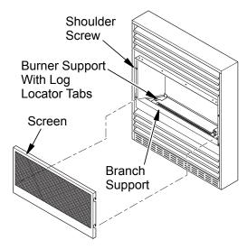
Figure 2 - Removing Screen
