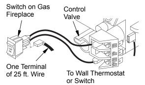
Figure 29 - Connecting Wire Terminals
