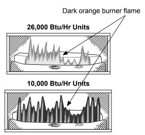
Figure 41 - Incorrect Burner Flame Pattern
