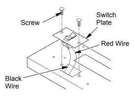
Figure 28 - Switch Plate and Wiring Harness
