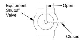
Figure 25 - Equipment Shutoff Valve
