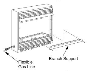
Figure 23 - Removing Branch Support From Fireplace
