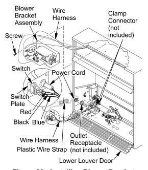
Figure 20 - Installing Blower Bracket Assembly
