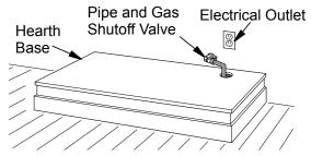
Figure 11 - Placing Hearth Base Against Wall
