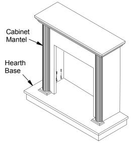
Figure 12 - Installing Cabinet Mantel onto Hearth Base
