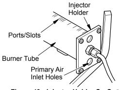
Figure 42 - Injector Holder On Outlet
