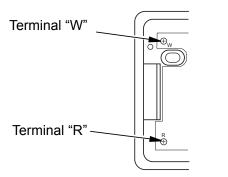
Figure 31 - Thermostat Base Terminals "W" and "R"
