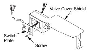
Figure 18 - Installing Switch Plate to Valve Cover Shield
