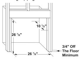
Figure 7 - Rough Opening for Installing in Wall
