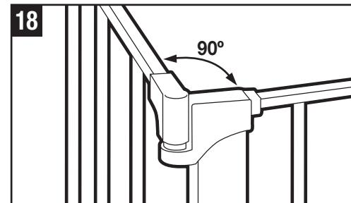
**18** Hold Open Feature – By opening the door to a 90° or greater angle, it will stay open until it is pushed closed.
