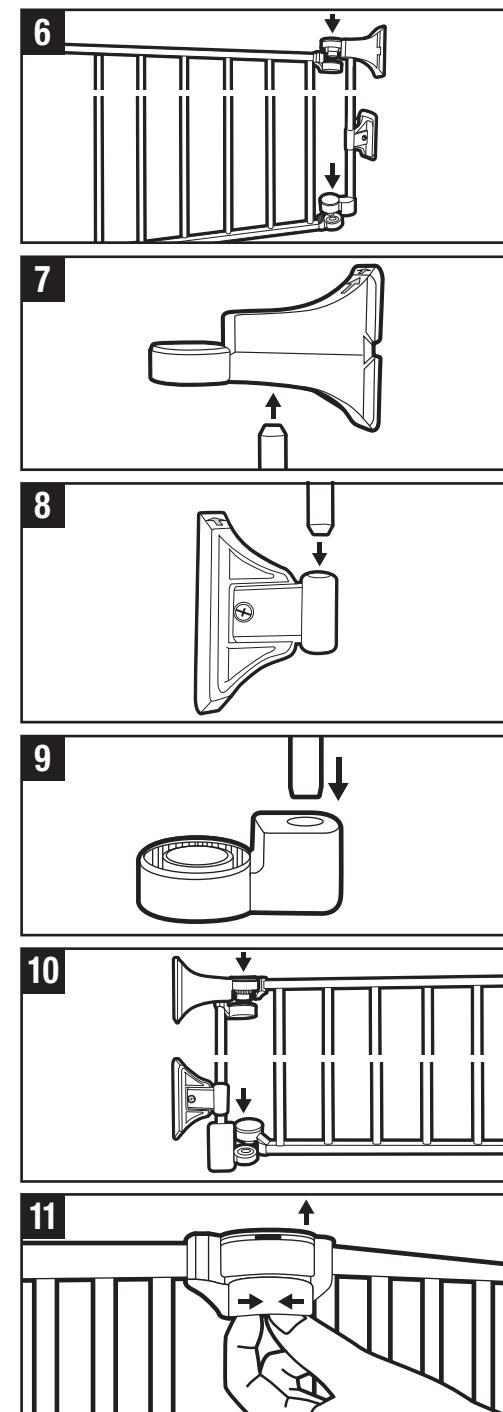
**6** Attach bar assembly to receiver of end gate section.
