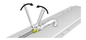
• Attach flex line from the burner to gas valve as shown below. Use two Wrenches to secure connection.
