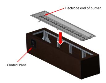
Orient burner so that the electrode is nearest to the control panel in order to make CF-SPARKER box connections.
