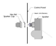
Read and understand your Crystal Fire owner's manual before beginning burner hookups or using the device. <u>Do not use Teflon tape or pipe dope on flare fittings.</u>
