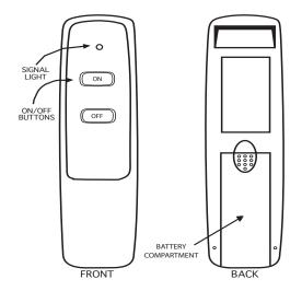
The transmitter operates on a 12V (A23) battery that is included. Install the 12V battery supplied with the unit into the battery compartment. It is recommended that ALKALINE batteries always be used for this product. Be sure the batteries are installed with the (+) and (-) ends facing the correct direction.
