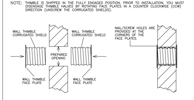
AFTER FRAMING THE PROPER SIZED OPENING, INSERT THE TWO HALVES OF THE THIMBLE FROM OPPOSITE SIDES OF THE WALL AND ENGAGE BY ROTATING THE FACE PLATES IN A CLOCKWISE DIRECTION (SCREW TOGETHER THE CORRUGATED SHIELDS)
