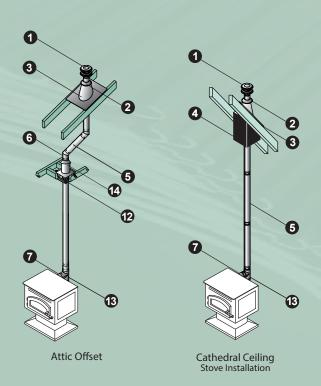
Refer to the Typical Secure Pellet Installations diagram, on the opposite page, to be familiar with some of the standard Secure Pellet installations and the required component parts.
