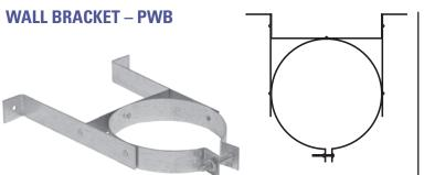
Used to provide lateral support while maintaining proper clearance. Recommended spacing is 6 ft. between bands above the starting point.
