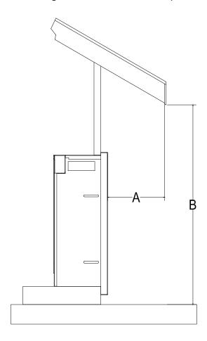
The overhang(A) must extend at least 1/2 the roof-line height. Height is measured from the base of the fireplace.
