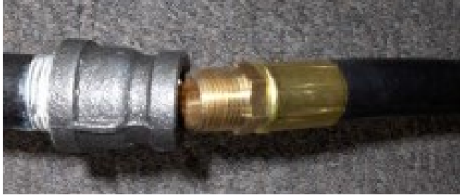
Figure 14: Gas Hose Connections
