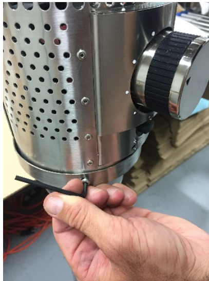
Figure 36: Hand Tighten Heater Head
