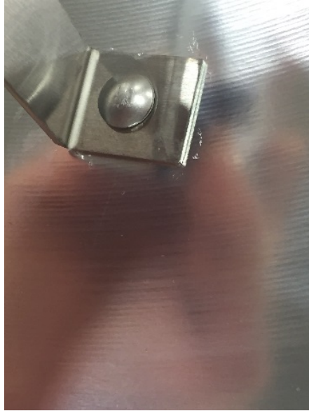
Figure 38: Place Reflector onto Heater Head
