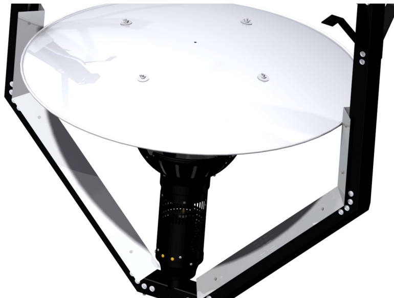
Figure 23: Install Heat Shields
