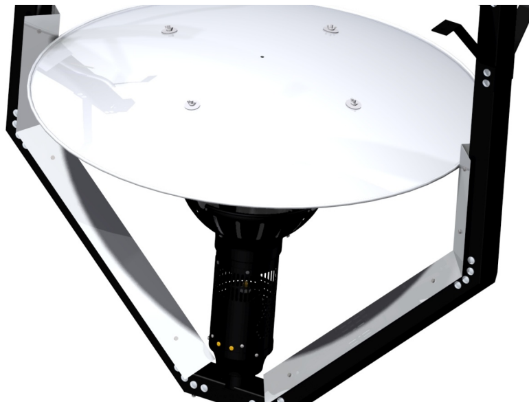
Figure 23: Install Heat Shields
