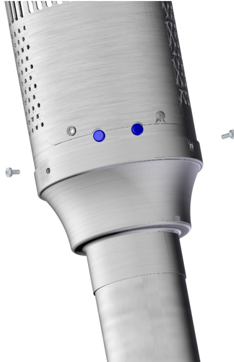
Figure 10: Burner Head Installation
