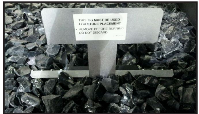
Figure 9.9 Rock Placement Jig
