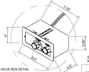
SPARK IGNITION BY AA BATTERY MATERIAL: 304 STAINLESS STEEL
