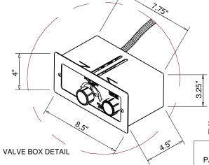
SPARK IGNITION BY AA BATTERY MATERIAL: 304 STAINLESS STEEL
