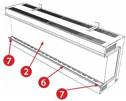
**Step 1** - Remove the 2 screws (item 7) that secure the front glass bottom retainer (item 6) to the fuel bed (item 8).
