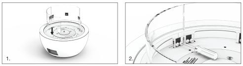
2. The round frameless glass installations are subject to tolerance and alignment issues. Please ensure that the glass screens have been properly pushed down into position and are not leaning outwards. If there are still alignment issues please adjust the screws where necessary with a Philips screw driver.
