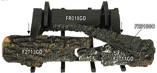
Place the FR018GO under the pedestals. Pull it forward until the front edge touches the front logs. This will create the heat chamber needed to help the logs glow and radiate heat.
