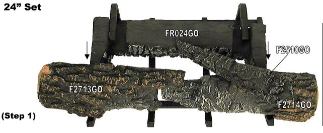
Place the FR024GO under the pedestals. Pull it forward until the front edge touches the front logs. This will create the heat chamber needed to help the logs glow and radiate heat.
