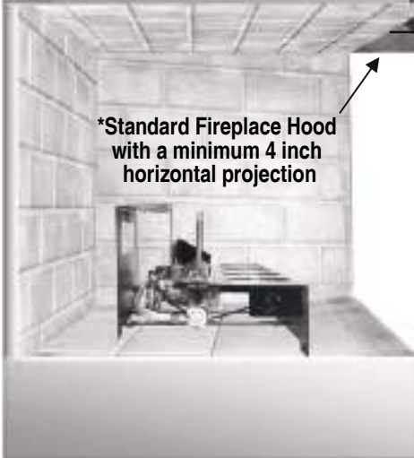
Distances from Top of Firebox Opening to Underside of Mantel
