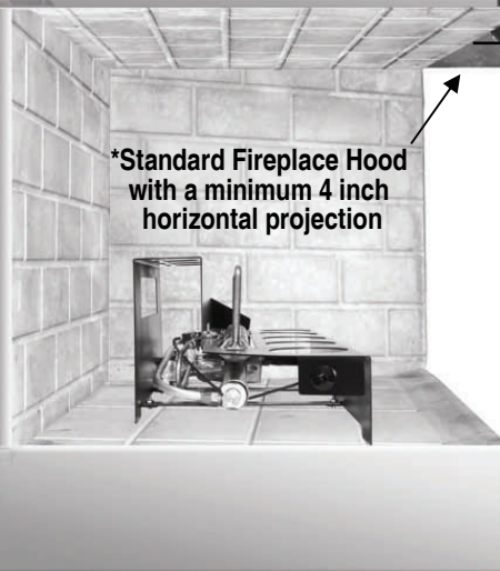
Distances from Top of Firebox Opening to Underside of Mantel
