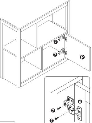
If necessary for correct door alignment, it is possible to adjust the hinges. See diagrams below:
