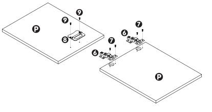
Hang the **Door (**) by attaching the **Hinges (**) to the inside right wall of the cabinet on the **Bottom** Shelf. For each Hinge, insert 4 Screws 🕑 through the eyelets of the hinge arm and into the holes on the inside wall as shown.
