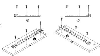
Insert Cam Lock Nuts ② into the corresponding holes above the installed Cabinet Runners on each Side. Rotate each Cam Lock Nut so the arrow (at one point of the Phillips head cross marking) points toward the adjacent hole in the edge of the panel as shown.
