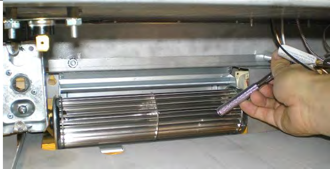
3. Hook Fan onto Studs. Replace and tighten nuts
