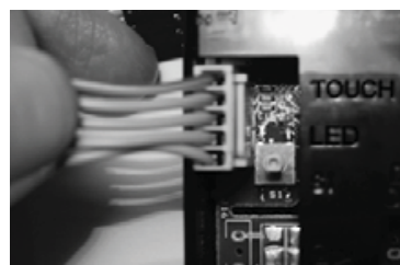
Figure 20 - Connecting end of Touch Pad Cable
