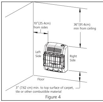
For convenience and efficiency, install the heater:
