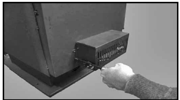
Figure 18: Installing the blower.
