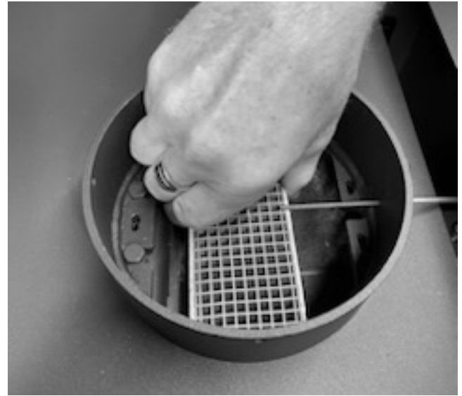
Figure 5: Position over combustor bracket.
